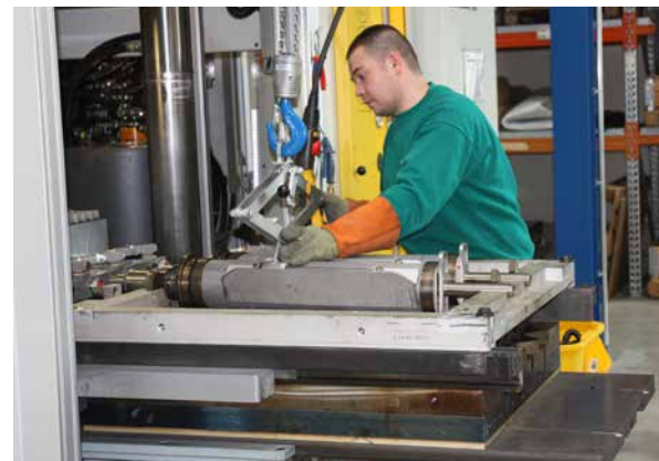
Injection moulding machine for iFD-stators®
