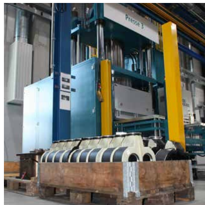
Press with casing liners for TORNADO® T2
